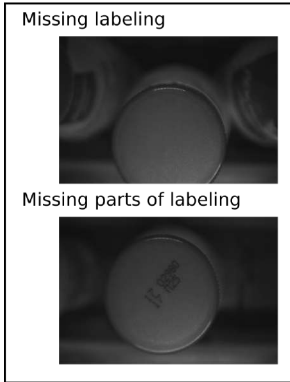
Figure 4. Main marking defects
