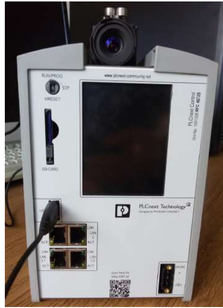
Figure 3. Controller RFC 4072S with connected camera DFK 22AUC03
