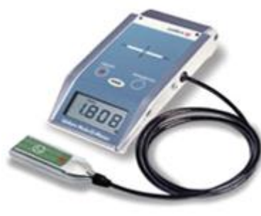
Figure 4. – Image of the Unfors mobile device
