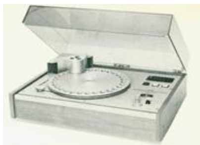
Figure 3. – Thermal flash disk irradiation device
