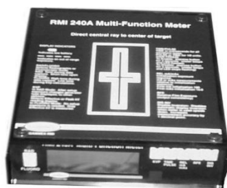
Figure 7. – X-ray measuring device RM 240
