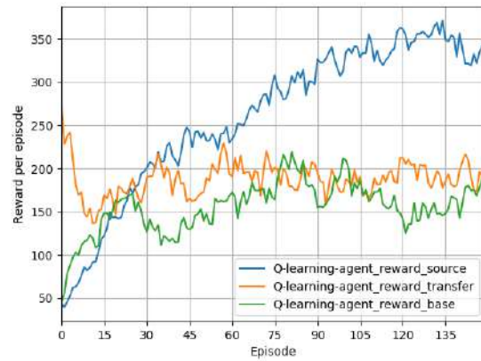
Figure 4: The asymptotically best performing algorithm of these three is the source algorithm which is in full agent-space (type A), its experience is transferred to the target algorithm with limited agent-space (type B) which shows a better starting efficiency and the worst performing algorithm is a type B agent without transferred experience that is a baseline for comparison. The source and target algorithms use argmax for action selection.
