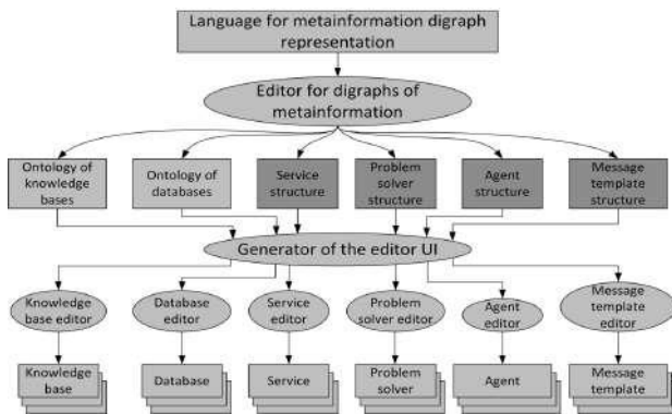
Figure 3. Usage of the development toolkit for creating information and software components of intelligent services.
