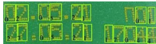
Figure 7. Detected digits in marking
