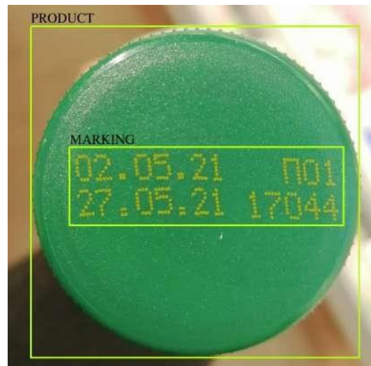
Figure 6. Detected product and marking
