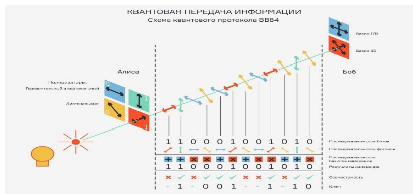
Figure 1. The scheme of the quantum protocol BB84
