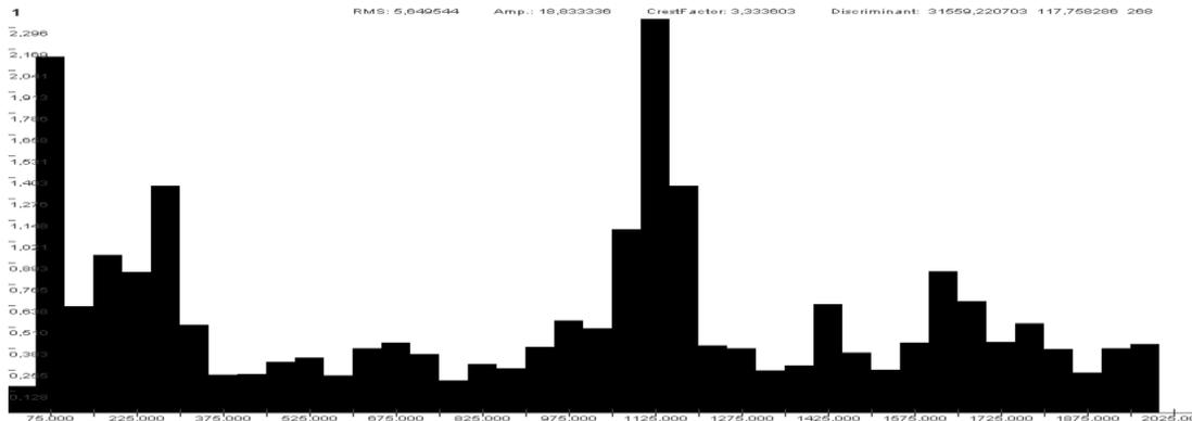
Figure 8: Band spectrum of vibration signal during turbine emergency state.
