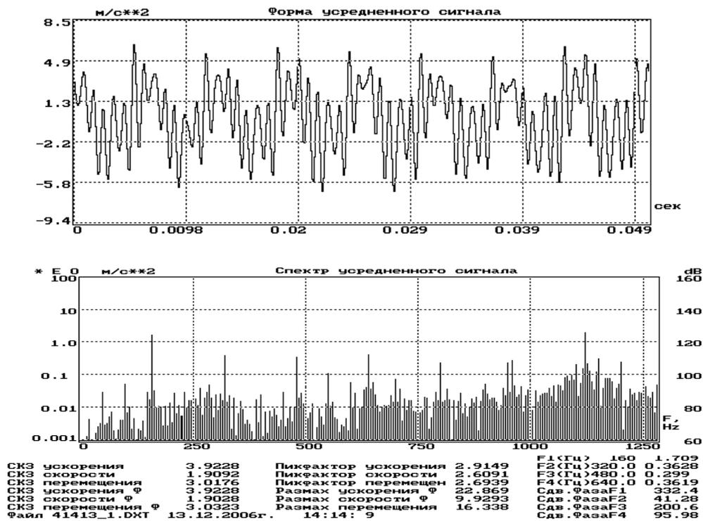
Figure 4: Vibration signal, averaged in the time domain synchronously with the frequency component of 160 Hz, turbine shaft speed, during normal operation
