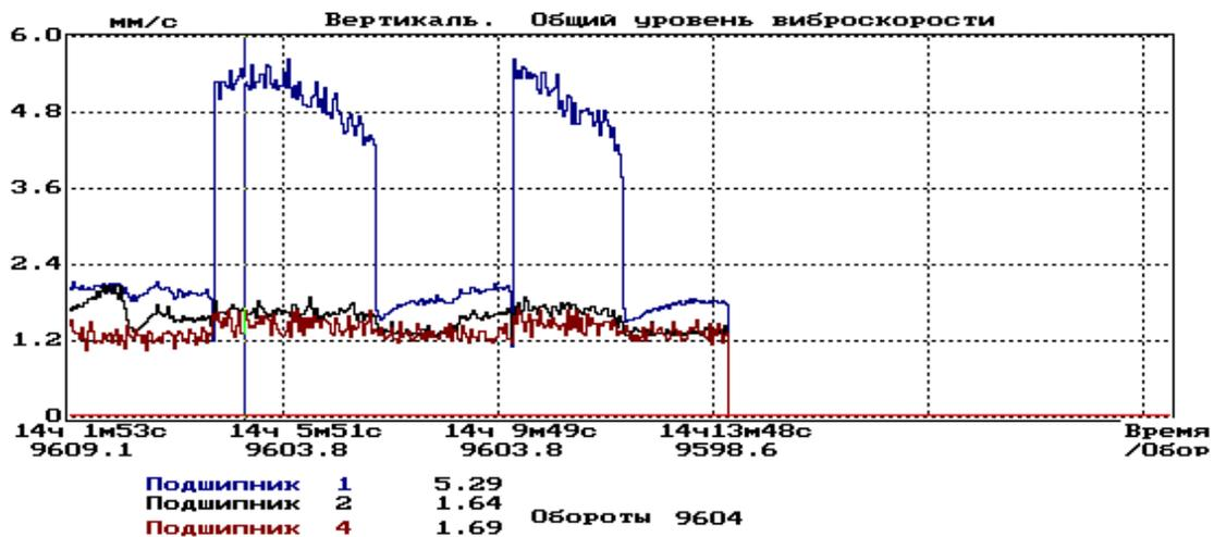
Figure 1: Change in RMS vibration velocity when changing the operating mode of the DGA.
