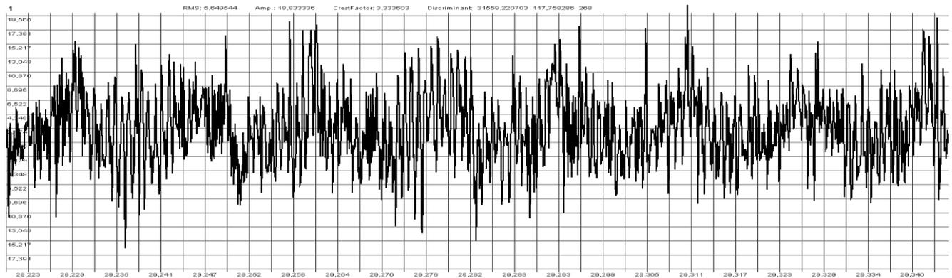
Figure 5: Temporary realization of a vibration signal in an emergency condition of the turbine.
