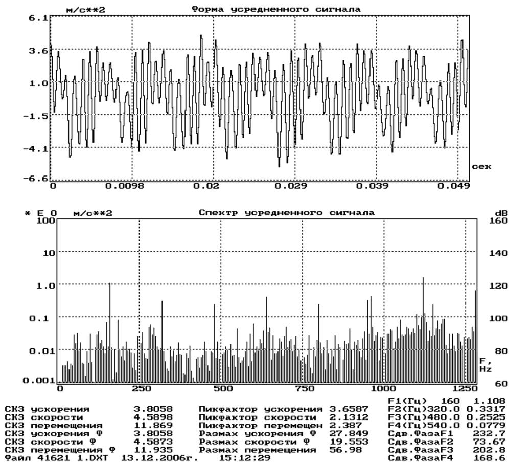
Figure 9: Vibration signal, averaged in the time domain synchronously with the frequency component of 160 Hz, turbine shaft speed, in emergency operation
