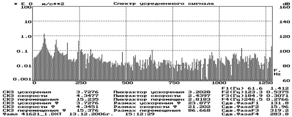
Figure 10: Vibration signal, averaged in the time domain synchronously with the frequency component of 62 Hz, basic disturbance frequency in emergency operation
