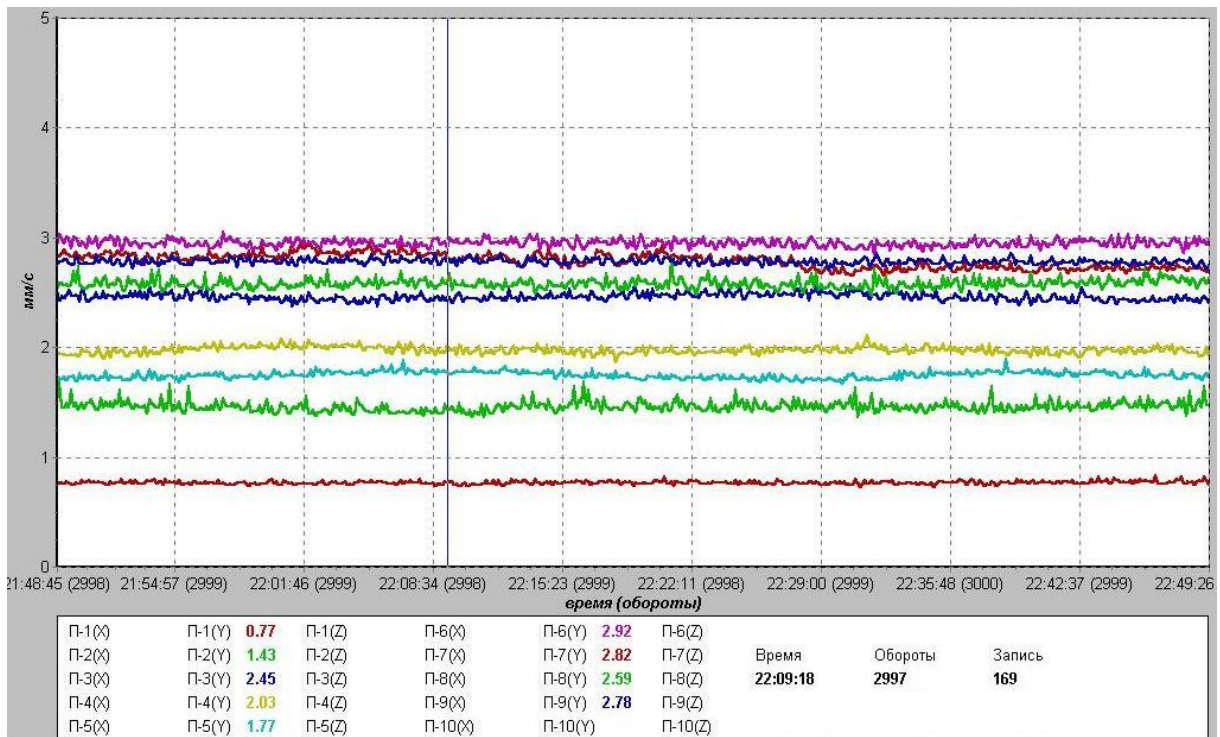
Figure 2: RMS trend of vibration velocity (vertical) of bearing supports turbine set during normal operation (abscissa axis – time (revolutions per minute) ; ordinate axis – vibration velocity, mm/s)
