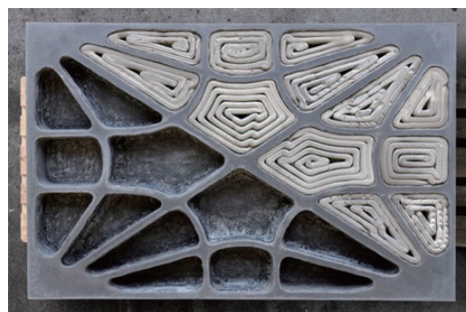
Figure 5. Foam 3D printing inside concrete construction [9]
