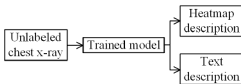
Figure 13. Operation schematic of the CXR-based decision support system under development.
