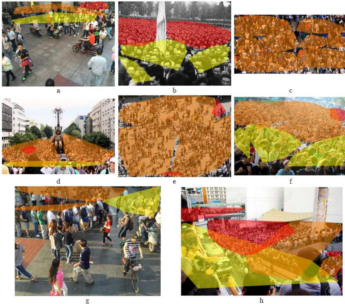
Figure 4. Semantic segmentation of crowds of different types: regular crowds with no attention (a, b), uniform crowd with regular attention (c), diverse crowd containing groups with increased interest (d, e), diverse crowd with a spreading group with interest (f), crowd with a queue (g), crowd with a close cluster (h)
