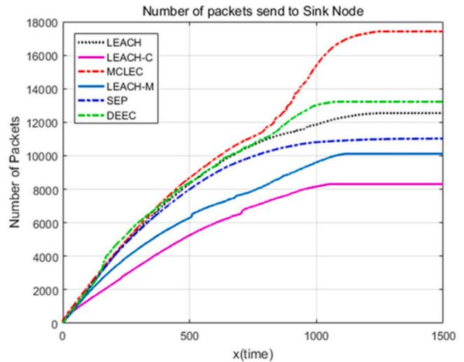
**Fig. 10.** Packet to sink node comparison chart.
