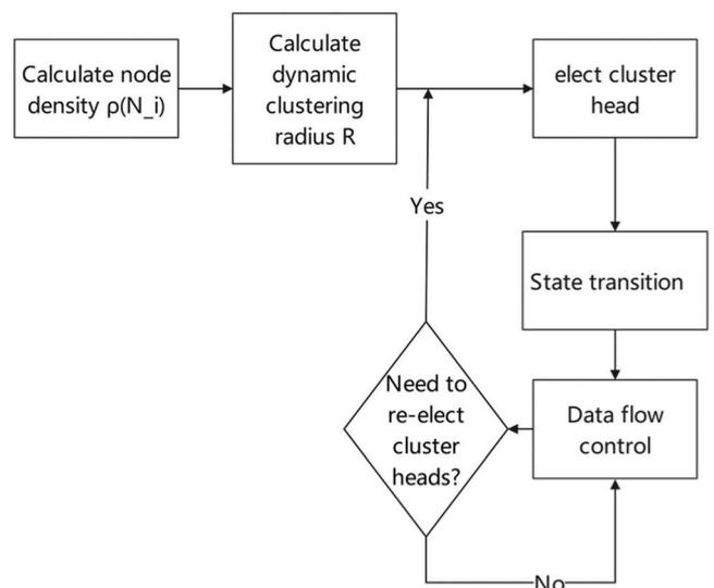
Fig. 4. Flowchart of FITNESS AND NODE DENSITY CLUSTERING MECHANISM IN MCS.
