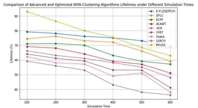
Fig. 17. Comparison of advanced and optimized WSN clustering algorithms lifetimes under different simulation times.
