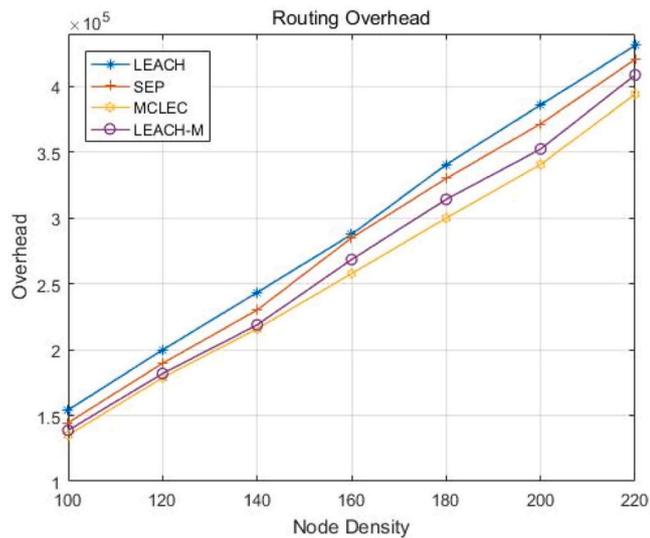
Fig. 15. Routing overhead comparison.
