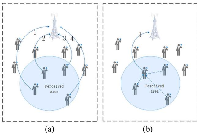
Fig. 3. A comparison of the two data transmission modes. (a) Data transmission by traditional group perceptive network. (b) Data transmission by cluster group perceptive network.
