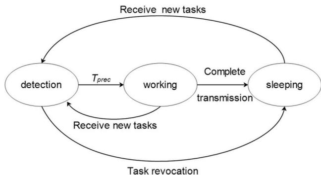
Fig. 5. Node state transition diagram.
